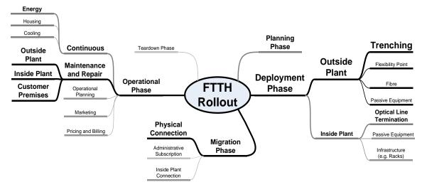
Figure 5: Breakdown of the cost (estimated) of a FTTH rollout with focus (size and weight) based on the impact of the part on the final cost
